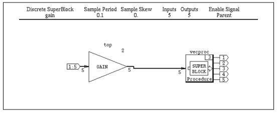
Figure 6-7. Vectorized Procedure Interface
